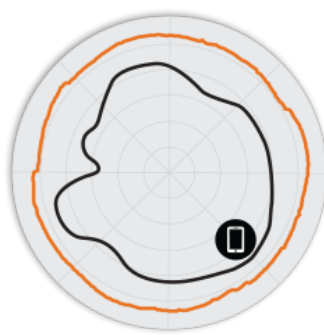
Figure 3. R850 5GHz Azimuth Antenna Patterns
