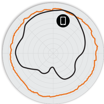
Figure 2. R850 2.4GHz Azimuth Antenna Patterns
